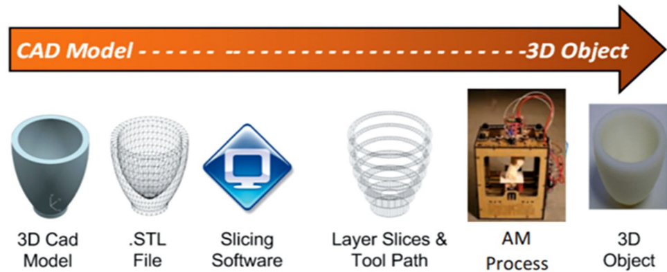
Fig. 3 Generalized 3D-printing process [33]
