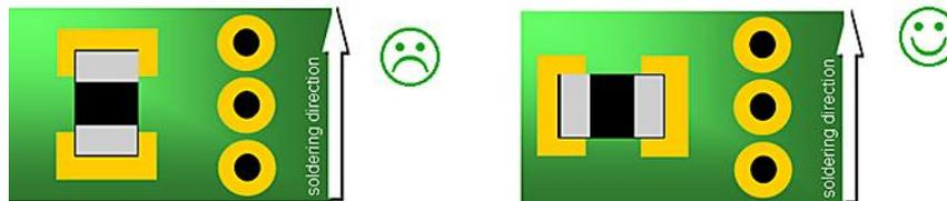
**Figure 6 – Alignment of neighbouring SMD components**
