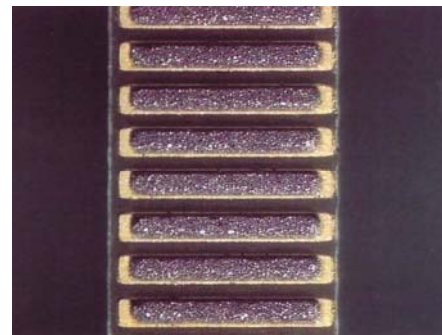
Solder paste with good gel system
