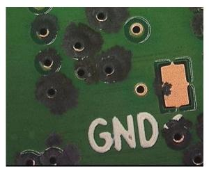
Figure 4: Corroded Cu with OSP finish
