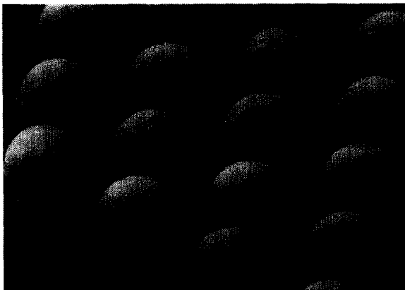
Figure 15 SEM of solder bumps utilizing fluxless soldering method [27].
