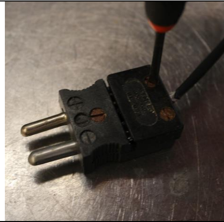
Attach T/C Cover As Shown.
