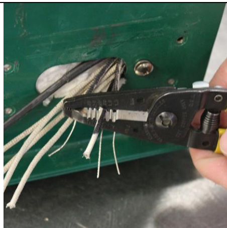
Trim to expose 1" of each wire. As shown.
