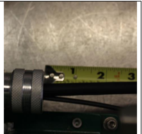
Measure Electrical wire 17 inches from cord grip.
