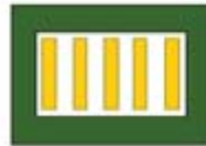
Windowed Solder Mask
