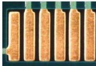
Windowed Solder Mask
