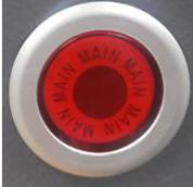
A circular lamp with a red lens and a silver metal ring. The lens has the words "MAIN POWER" repeated around its perimeter.  | <b>Main Power Lamp</b>         | Displays whether the main power is on or not.                                                                                                                                                                                                                                                                         |
