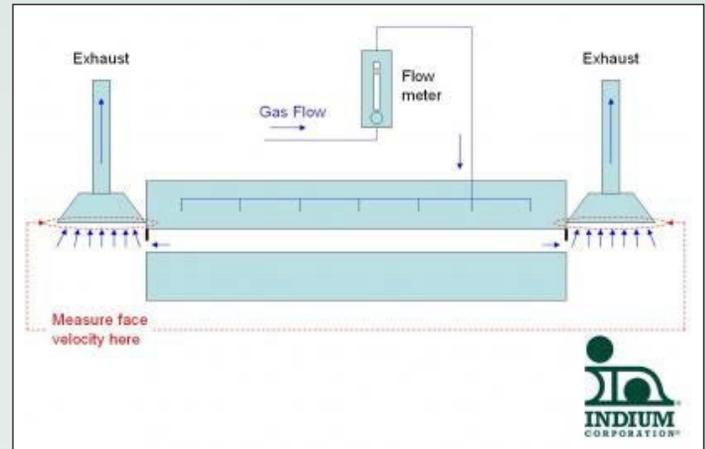
**One final note:** Inert or “nitrogen” soldering really should be renamed “low oxygen level” soldering to place emphasis on the control variable: the ppm oxygen ( $O_2$ ). From an engineering perspective, it IS a critical control variable, and ppm levels within reflow ovens should be measured on a continuous basis.
