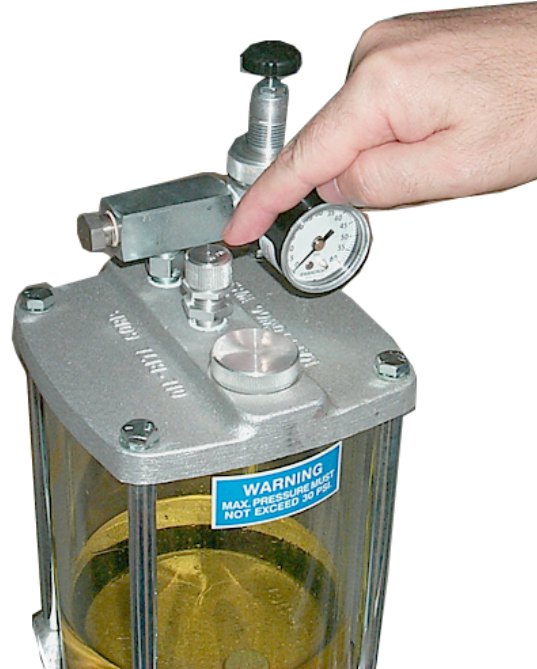
Figure 33: Pointing to Bleeder Valve on Top of Reservoir — DO NOT ADJUST
