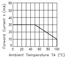
Fig. 3 FORWARD CURRENT DERATING CURVE
