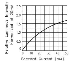
Fig.4 RELATIVE LUMINOUS INTENSITY VS. FORWARD CURRENT
