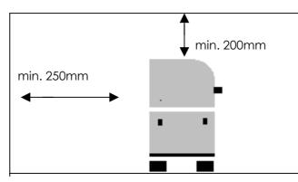
On top of the housing is an integrated fan. It is used for cooling the housing and enables convection heating. Never block this fan by putting something on top or by not respecting the minimum distance. Level the oven on the floor by using the integrated feets.
