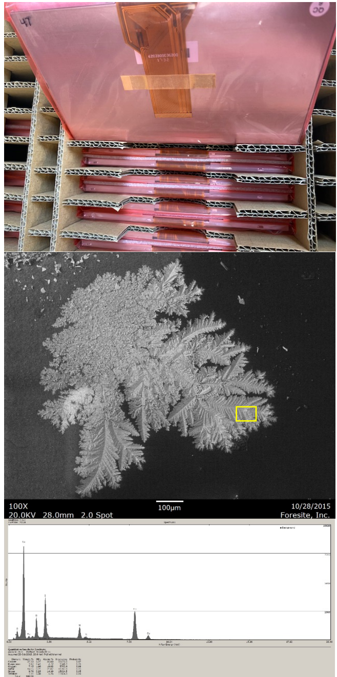
Figure 14/15/16: Display in ESD Bag, sample location for EDS elemental analysis which shows sulfur at 16.5 wt% and nothing present in the ESD Bag but at 18.9% in the cardboard separator.
