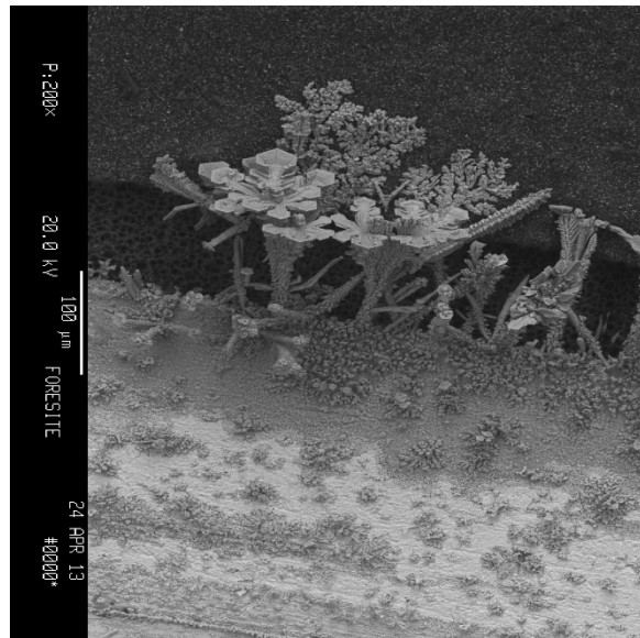
Figure 9: Immersion silver trace exposed to a rubber band at Foresite for 48 hours at 60C in sealed bag
