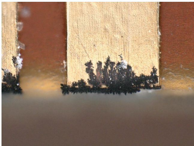
Figure 13: Flex circuit ENIG finish over copper inside ESD bag next to cardboard separators for 1 year inside box.
