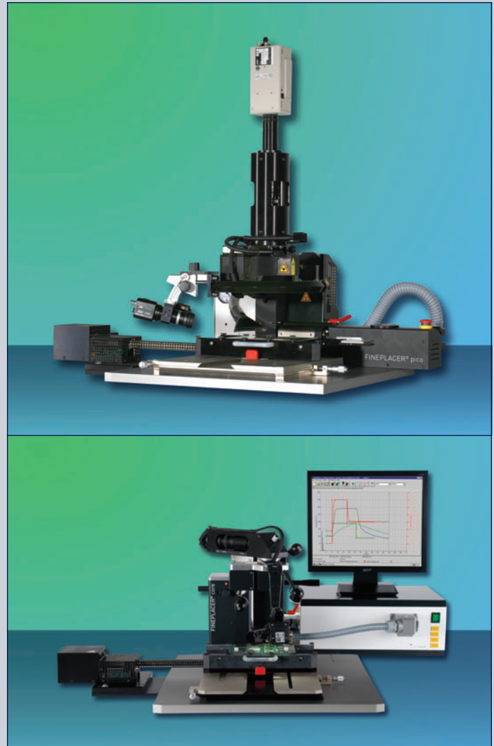
Figure 1: Examples of flip chip rework stations. Features for flip chip rework include placement accuracy of better than 10 microns and precision thermal management.
