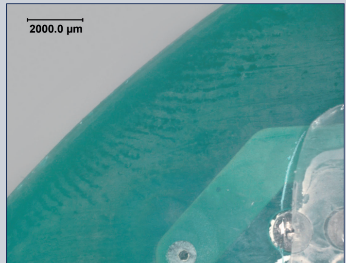
Figure 2: The oils from this fingerprint contributed to poor adhesion of the conformal coating and led to the corrosion seen in Figure 1.
