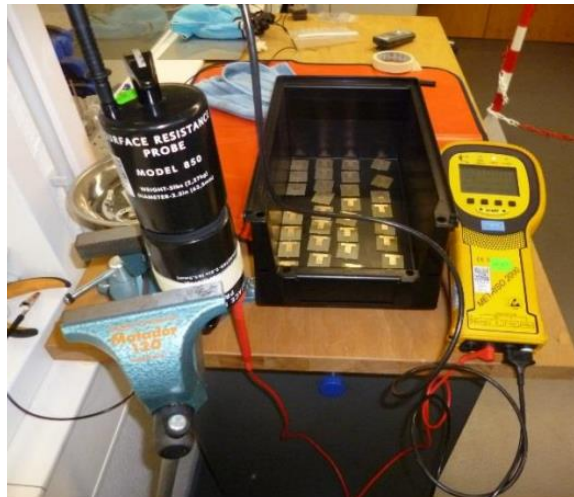
Figure 5 - Test circuits are sandwiched between test probes for resistance test
