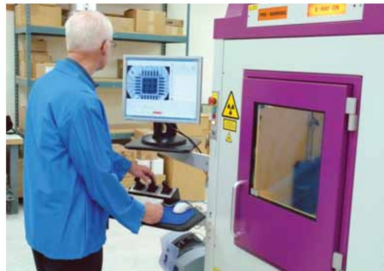
The micro-focus X-ray system is used for quality verification, troubleshooting and repair.
