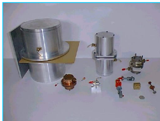
Figure 2 – LCP samples supplied and examples of cavities used for the characterization
