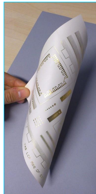
Figure 8 – Second breadboard : double sided board on 100 microns thick LCP
