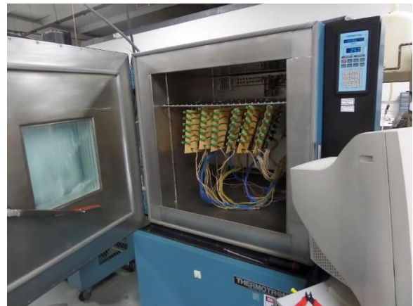
Figure 11 – Environmental Chamber with Socketed Boards
