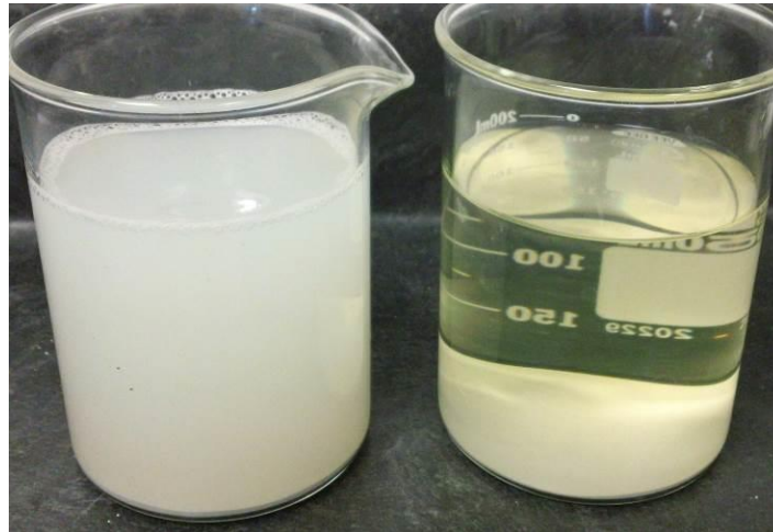
Figure 8 - Solder paste mixed with water. Water washable (left) vs. water soluble (right)
