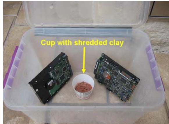
Figure 11. Mild clay test setup. 30g of shredded clay is placed in a cup and heated inside the enclosed container. Samples are placed in after heating.
