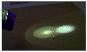
Fig. 12. Inspection of a sealed bag of polyimide prepreg showing UV fluorescence of particulate contamination.
