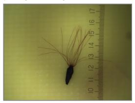
Fig. 8. Top view of a laminate after etching of copper cladding, showing a plant seed embedded in the dielectric material, probably carried into the clean room on clothes of personnel. The scale is in mm.
