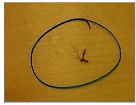
Fig. 9. Top view of a prepreg showing an embedded insect.
