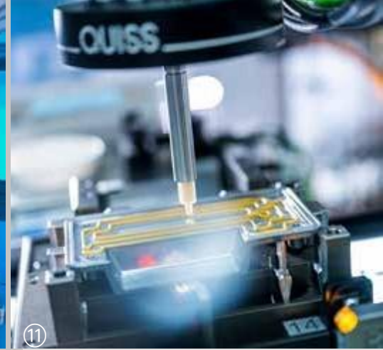
Fig. 9: DosPL DPL2001 – highly precise application from the smallest volumes to the µl range.
