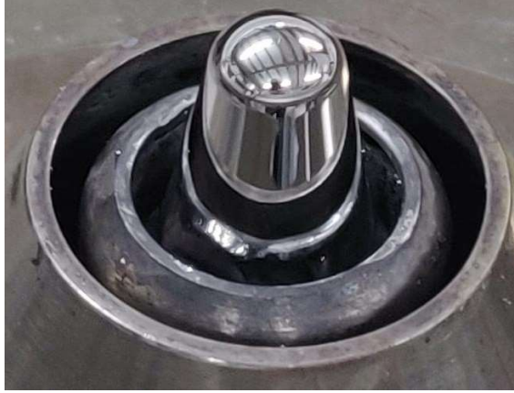
Figure 3. An example of a wetted nozzle.
