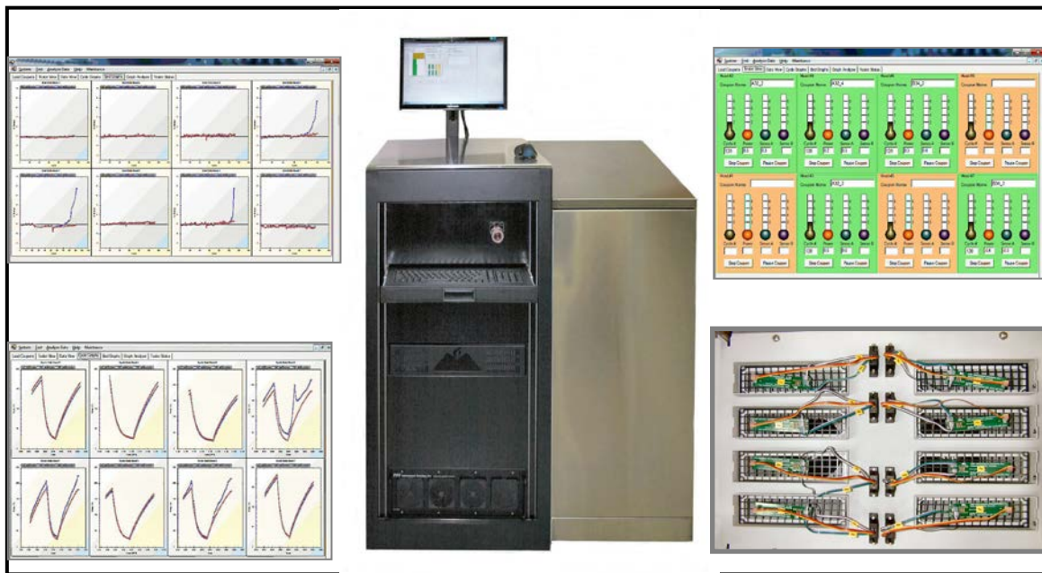
Figure 2 –IST Tester, Eight Head with Coupons, Three Screen Shots
