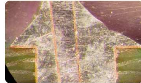
SACX after cycling – no cracks
