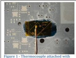
Figure 1 - Thermocouple attached with Kapton® tape
