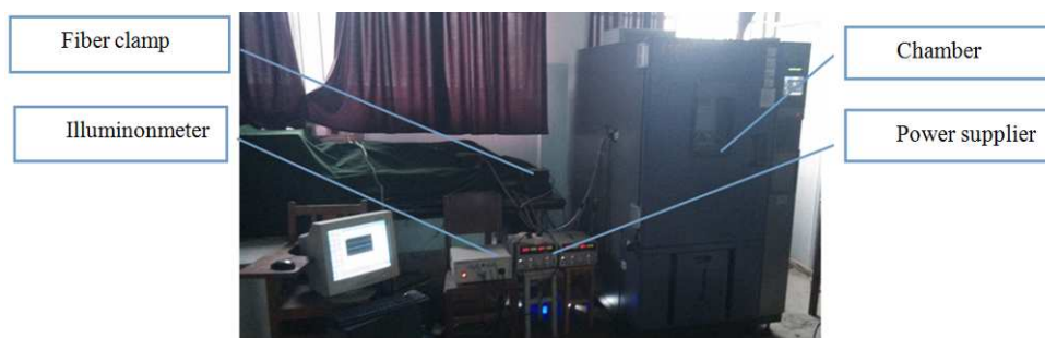
Fig. 2 Aging test system with online LED luminance measurement
