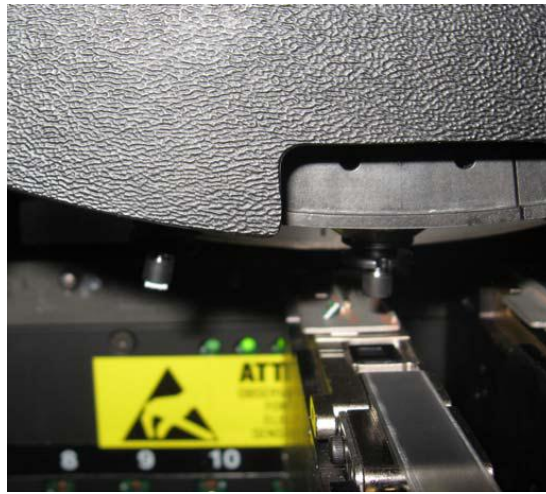
Graphic 3 Part not releasing during placement
