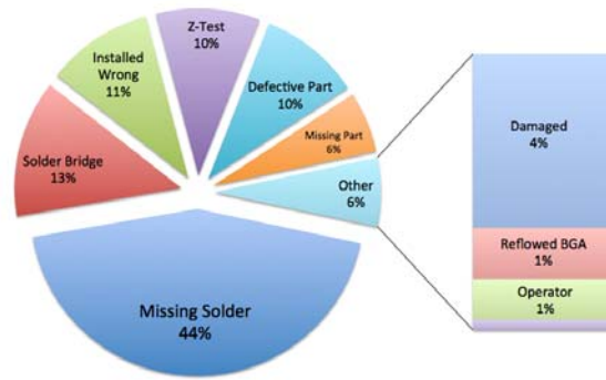
Figure 3. Defect Classifications across ICT and Functional Test
