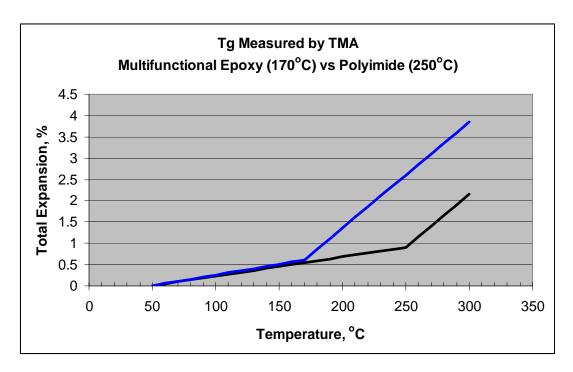
One of the most common results of the softening of the resin at its Tg is that it becomes easily smeared during drilling. With conventional FR4 the heat generated at the cutting surfaces of the drill is usually sufficient to cause smearing. In addition, when resin is heated above its Tg, either in use or during processing, it will cause substantial reduction in bond between the resin of the laminate and its copper foil cladding, resulting in pad lifting and other problems with surface features.
