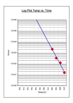
There are many ways to evaluate this. Underwriters Laboratories develops a thermal index (Arrhenius plotting of time vs. temperature) for materials which is the mathematical extrapolation of data from a four temperature accelerated aging evaluation to a temperature at which the material will operate for 100,000 hours and still retain at least 50% of its original physical or electrical properties.
