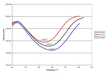
The "integrated flow" is an expression of the total area under the flow curve (remember that flow is proportional to the inverse of viscosity, or 1/Eta\*) over time and gives an idea of the total flow achievable by a system. Integrated flow allows a convenient comparison of prepregs in terms of total flow.
