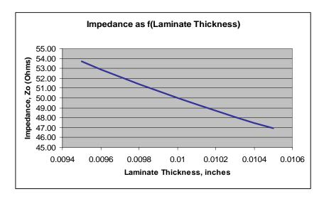
The effect of either, laminate thickness (Note: this is equally true for inner layer dielectric spacing!) or line thickness and width, is greater than that of dielectric constant, which is an inverse square root function. (see charts below showing impedance as a function of normal
