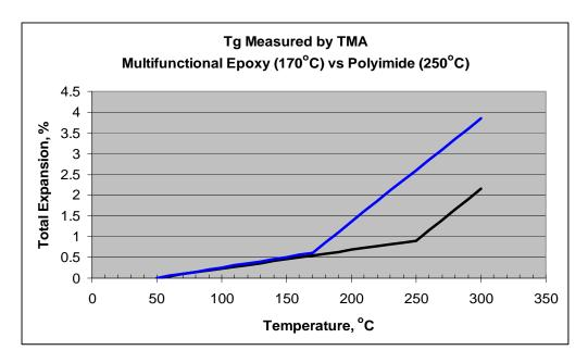
plated in holes, the extra expansion above the Tg is often responsible for PTH copper cracking during processing or rework. It may also result in "latent defects" that will show up later during normal in-service use.
