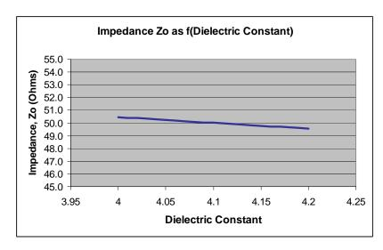
variation in dielectric constant and impedance for as typical polyimide product with nominal Dk of 4.1 and thickness of 0.010") These relationships will always be similar when considering the sources of impedance variation within a given system, regardless of the absolute values of the variables.
