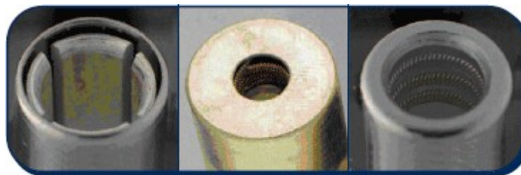
Figure 1-3: Shown left to right are Standard #4 socket contacts (4 contact bean springs), DCX CHOL/Methode (woven Kevlar), and ITT Canon/Methode (toroidal spring). The DCX and ITT contacts represent substantially higher current carrying capacity than the standard contact.
