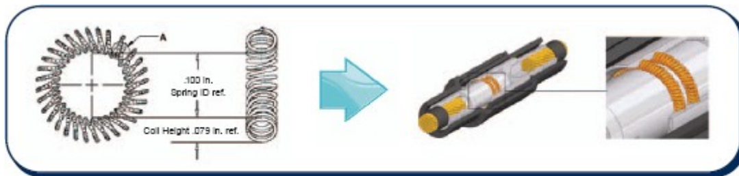
Figure 1-1: Bal Seal Corporation's toroidal spring concept. Each coil in the spring provides an additional contact point between the contact pin and the contact socket. Several such springs are inserted into grooves in the socket contact. When the pin is inserted, many contact points engage the pin.
